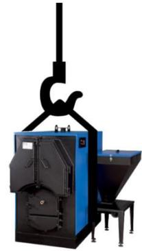
It is convenient to lift from the forklift stands or the carrying ring on the boiler. If the connecting ropes are to be passed under the boiler while lifting by crane, preventive measures should be taken against crushing the top of the boiler by the ropes. The boiler standing on the ground should be lifted directly without pulling with a crane. When transporting in cold weather, the boiler should not be lifted suddenly in case the rope freezes from the cold.
